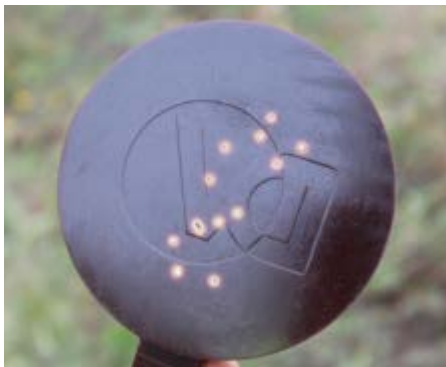
In cooler weather on day of testing, impacts displayed as yellow with a pinkish outline before fading back to black.
