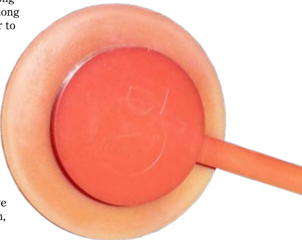
Half an hour later the lower target is turning yellow as it nears its maximum 40C maximum operating temperature.
